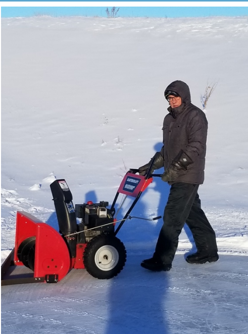
John Thiesen created a power scraper to maintain the pond skating and croicurl ice
